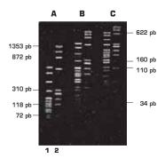
Novagel GQT Agarose gels in 1X TBE buffer. A-2%, B-3%, C-4% Markers: lane 1-pBR322 DNA. Mspl, lane-2-40x174 DNA.Haelll. Electrophoresis conditions: submarine gel, 2 hours, 4.5 V/cm. in 1X TBE buffer.
